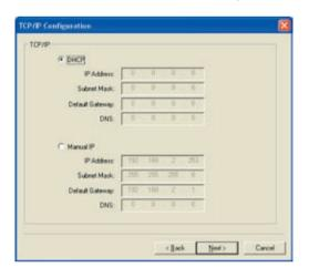
The Print Server by default will try to get an IP address from the connected Belkin Router running the Dynamic Host Configuration Protocol (DHCP) server and the following screen will appear.
